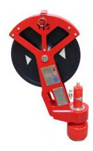
TIS Stuffing Boxes are designed to retain well pressure around moving and stationary slickline while guiding it into the top of the surface well intervention manifold.
