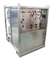
TIS Grease Injection Units are designed to introduce grease into a lubricator stack, typically for braided line applications, during well intervention operations.
