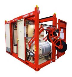
TIS Wireline Units are designed for controlled deployment and recovery of slickline, braided line and electric line from an open console or fully containerised unit, during well intervention operations.
