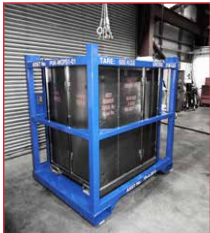
SKID FOR WELL CONTROL PANEL
