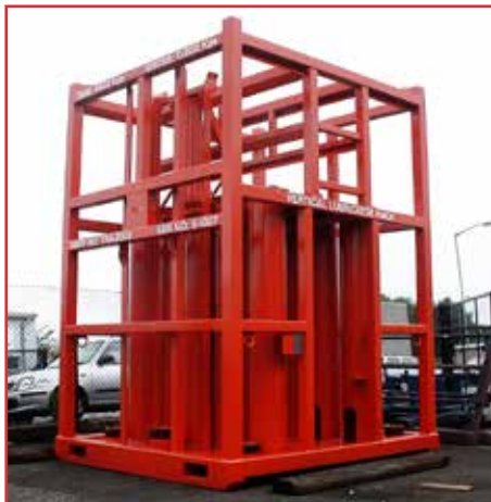
VERTICAL LUBRICATOR STORAGE SKID
