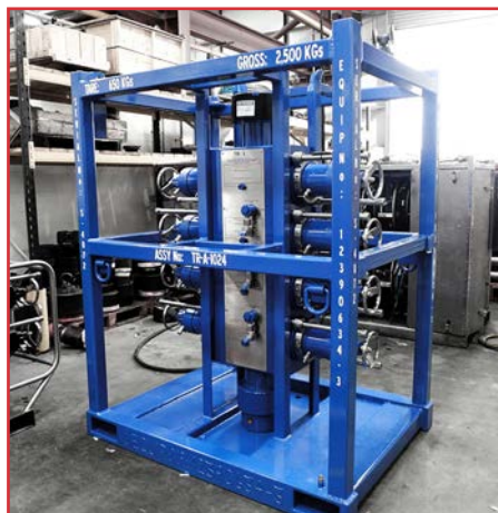
SKID FOR QUAD WIRELINE VALVE
